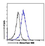
Flow cytometry analysis of paraformaldehyde fixed MCF7 cells (blue line), permeabilized with 0.5% Triton. Primary incubation 1hr (10 µg/ml) followed by AF488 secondary antibody (1 µg/ml). IgG control: Unimmunized goat IgG (black line) followed by AF488 secondary antibody.
